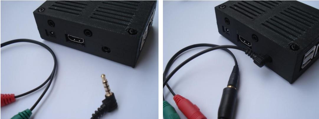
NOTE: Most PC headsets (if they have a 4 pin, 3.5mm TRRS connector) use the CTIA standard therefore will not work when plugged directly into the Pi-SDR IQ Plus. An OMTP to CTIA adapter cable is provided with the Pi-SDR along with a 4 pin TRRS splitter cable for headsets with separate MIC / PHONE TRS 3.5mm connectors.
