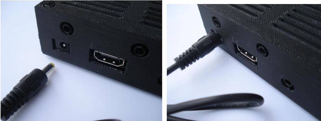
The user provided power supply needs to have three requirements, first to have a USB connector to connect with the provided power cable, second to be rated 5V 2.5Amp and finally to be 'quiet' in terms of electrical noise effects.
