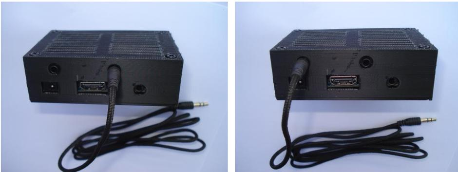
And one for Tx IQ connection, it should be connected to IQ-IN TX input of RS-HFIQ and to the left upper side connection of Pi SDR IQ Plus
