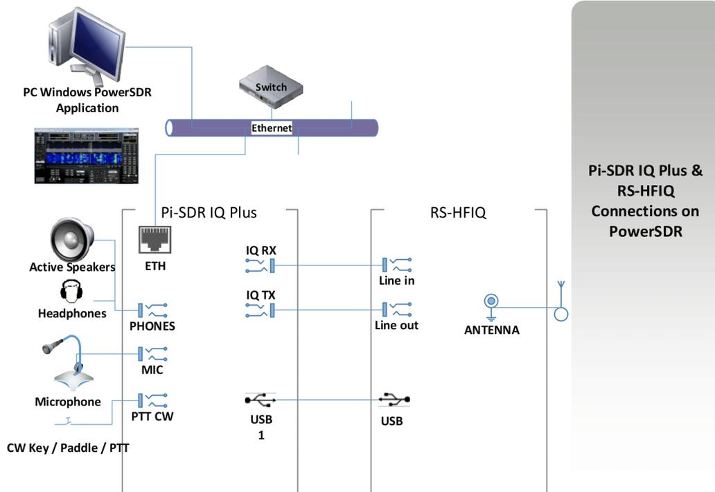
As the connection schematic indicates, we have to connect the Win/10 PC that executes PowerSDR to the local Ethernet network. Connection speed has to be at least 100MBps (100Base-TX).
