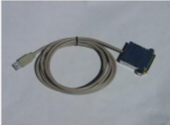
The USB to Parallel adapter eliminates the need for a parallel port interface on your computer. Unlike other off-the-shelf adapters, the FlexRadio Systems adapter implements all the data, status, and control lines for complete integration with existing parallel port hardware. For more information, see <http://www.flexradio.com>.
