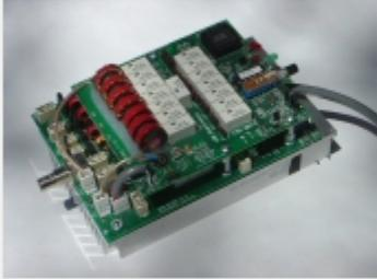
The integrated ATU allows the user to tune coax antennas with an SWR of up to 10:1. For more information, see <http://www.flexradio.com>.
